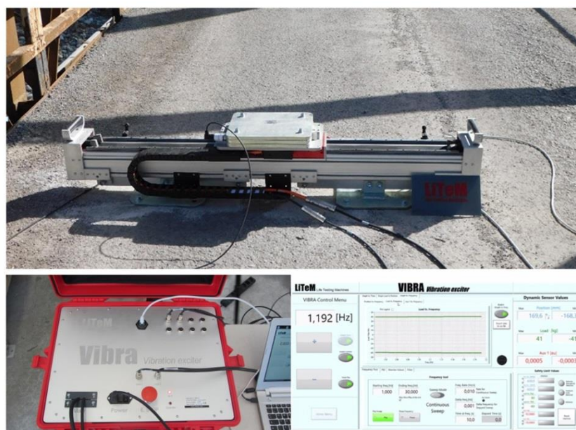
Fig. 5.3 VIBRA 9001 linear vibrodyne, controller and software – Litem - life testing machine
